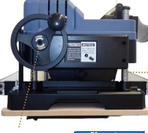
**Elevation Handwheel** Handwheel with lock knob design preventing from wheel self rotating.
